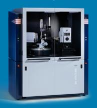
The G.L. Clark X-ray Facility is pleased to announce that our new diffractometer has arrived. The new instrument features the latest PHOTON-III detector, a third generation microfocus Mo source, a second generation diamond microfocus Cu source, and an Oxford 800 Plus cryostream. Please send us your crystals even if you think they will not diffract, the new detector and sources mean they just might have a chance.
