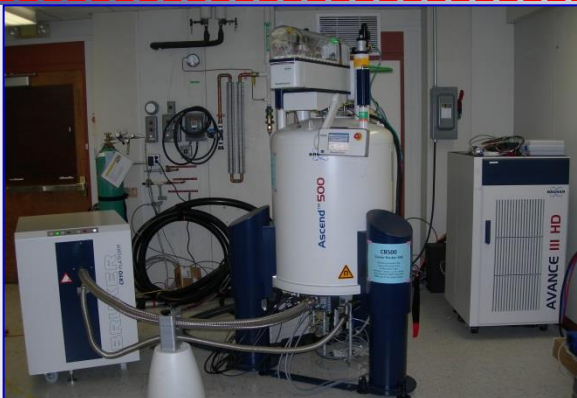
500 MHz: CB500 CryoProbe with 45 Nuclei
