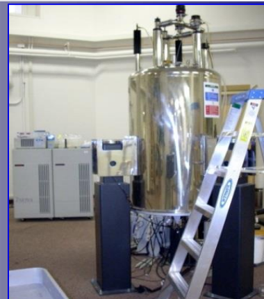
600 MHz: AutoX BB and HCN probes
