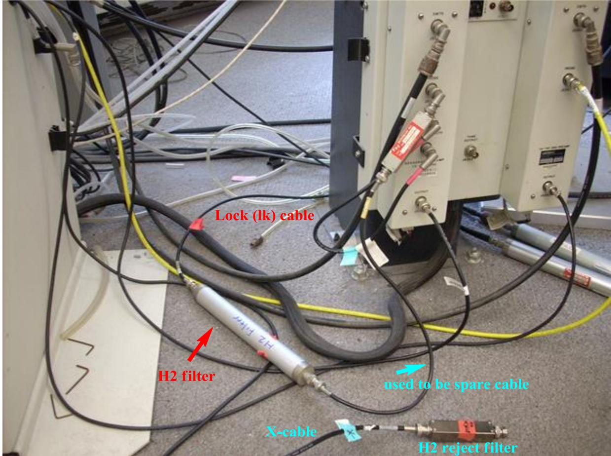
**Fig 2.** Configuration for deuterium cabling NMR on the UI500NB.
