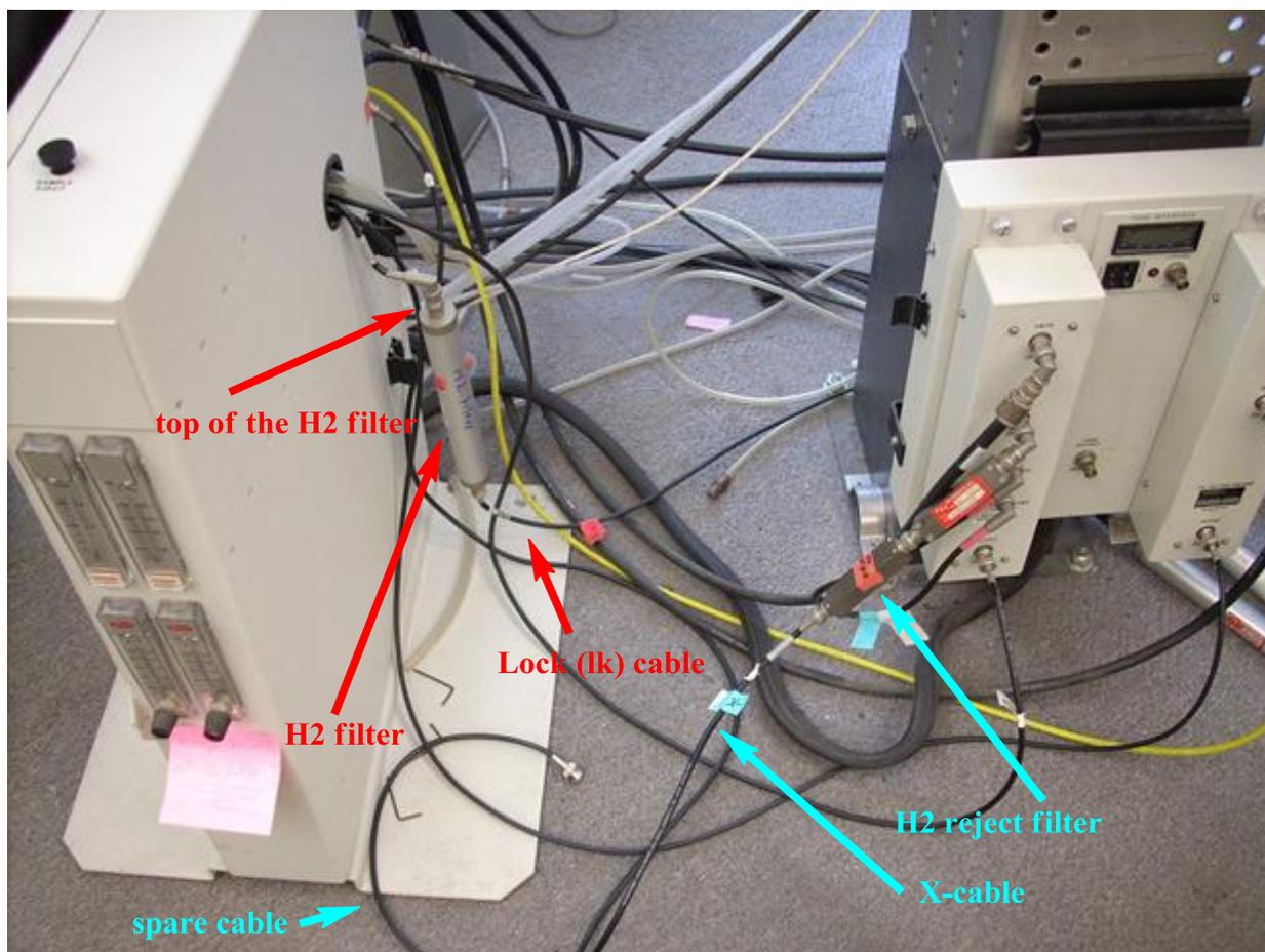
Fig 1. Original cable configuration of the UI500NB.
