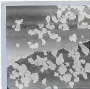
**Figure 4:** 110 x 110 nm STM image showing submonolayer coverage of a  $\alpha$ -SiW<sub>12</sub>O<sub>40</sub><sup>4-</sup> on an Ag(111) surface in 0.1 M aqueous H<sub>2</sub>SO<sub>4</sub>.
