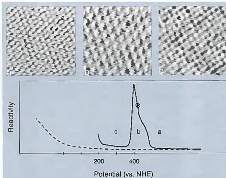
**Figure 2a:** AFM images (5 x 5 nm) of Bi up on Au(111) in 0.1 M  $HClO_4$ . a) Au(111) surface found positive of Bi up peaks. b) (2 x 2)-Bi adlattice found at +200 mV of bulk deposition. Atom-atom distance is  $0.57 \pm 0.02$  nm. c) Uniaxially commensurate rectangular Bi adlattice found at 100 mV. Atom-atom distance is  $0.34 \pm 0.02$  nm. **2b:** Reactivity plot of deposition stages.
