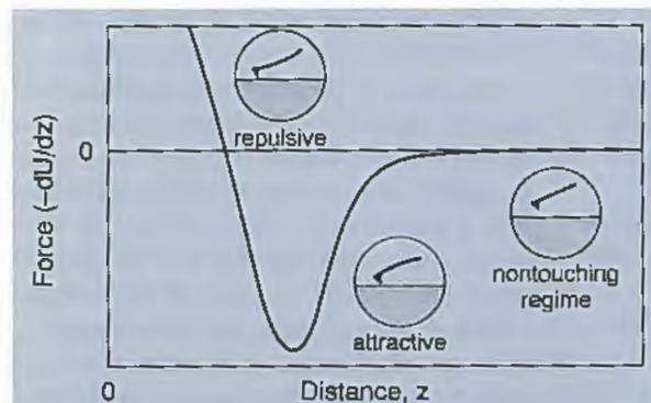
**Figure 1:** A force-distance curve. The insets show the tip curvature for (from left to right) tip in contact with the surface (repulsive interaction), tip and surface attracted (attractive interaction), and the non-touching regime (no interaction).
