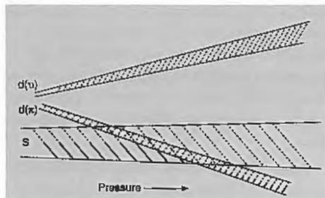
**Figure 2. Relative Energies of Energy Bands Arising from Atomic Level s, ds and dp Orbitals as a Function of Pressure** • Within each band, the solid diagonal lines represent the filled levels while the dashed lines indicate empty levels available for electrical conduction.
