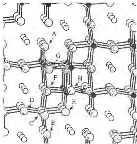
**Figure 2. Resolution of  $^{17}\text{O}$  NMR Resonances of Barium Dytitanate** • Shows that barium dititanate contains eight types of structurally distinct oxygens labeled A-H above. At high magnetic fields, seven of the eight  $\text{TaTi}_2\text{O}_6$  solid state  $^{17}\text{O}$  NMR resonances can be resolved.
