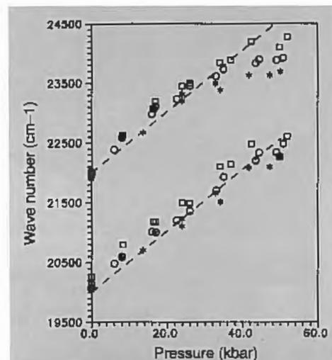
**Figure 4. Shift of the Blue and Green Emission Peaks with Pressure** • The shift of the blue and green emission peaks with pressure is essentially identical for all these materials with different degrees of doping. The dashed line shows the change of the energy difference between the highest filled band and the lowest empty band in ZnS. The emission energies increase in direct proportion to the change in the ZnS host material.
