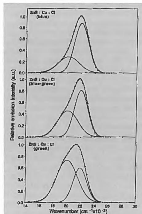
**Figure 3. Emission Spectra from Three Samples** • The blue emission from the Cl<sup>-</sup> donor to the Zn(II) acceptor is at  $\sim 22,500$   $\text{cm}^{-1}$ . The green emission (from Cl<sup>-</sup> to the Cu<sup>+</sup> acceptor) is at  $\sim 20,000$   $\text{cm}^{-1}$ .
